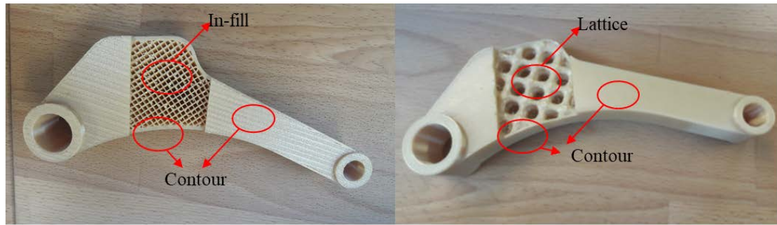
Figure 1. Types of inner structure: in-fill (left), lattice (right)
