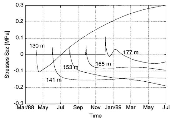
FIG. 2. Short-Term Stress Evolution for Different Elevations
