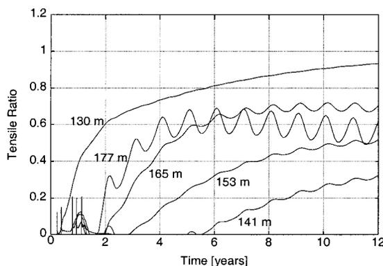
FIG. 8. Long-Term Tensile Ratio Evolution for Different Elevations with 3-Month Interruption
