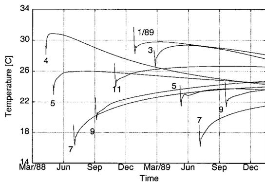
FIG. 10. Temperature Evolution for Different Elevations Slowing Construction Process
