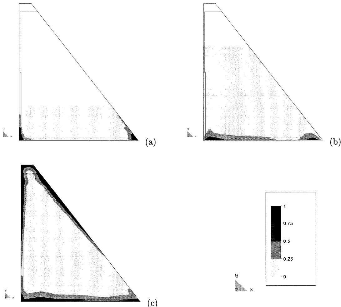
FIG. 5. Short-Term Evolution of Tensile Ratio; Corresponding (Months) Elevations Are: (a) (June 1988) 146 m; (b) (November 1988) 175 m; (c) (June 1989) 196 m
