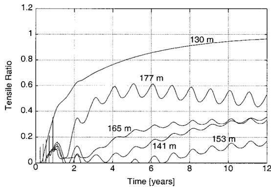
FIG. 4. Long-Term Tensile Ratio Evolution for Different Elevations
