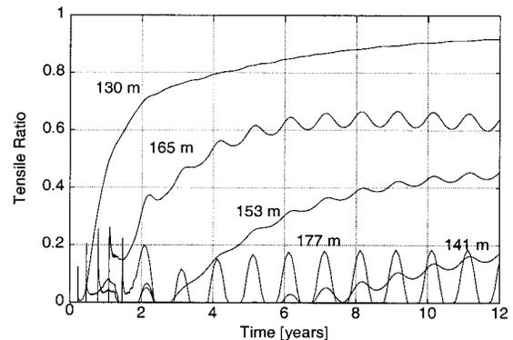
FIG. 11. Long-Term Tensile Ratio Evolution for Different Elevations Slowing Construction Process
