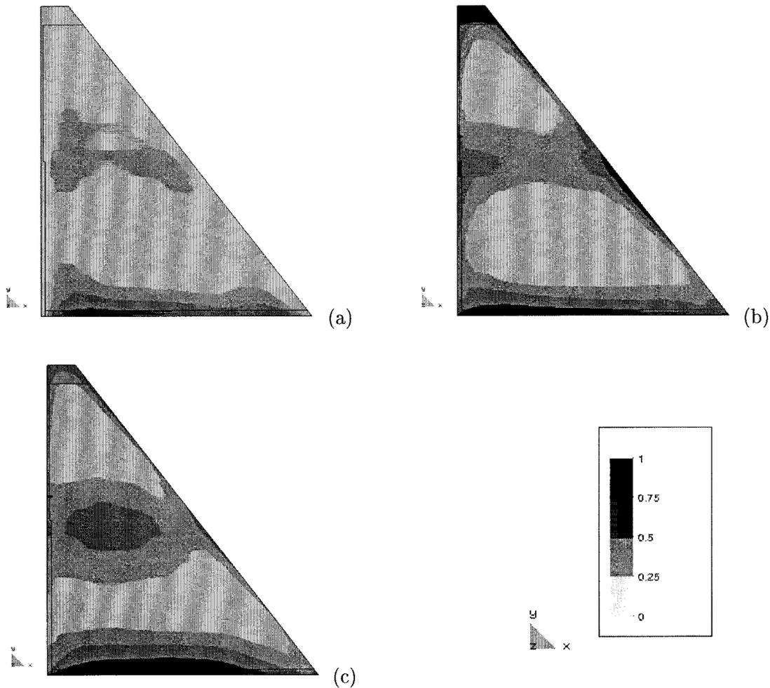
FIG. 12. Long-Term Evolution of Tensile Ratio Slowing Construction Process; Winter Distribution for: (a) 1990; (b) 1992; (c) 2000
