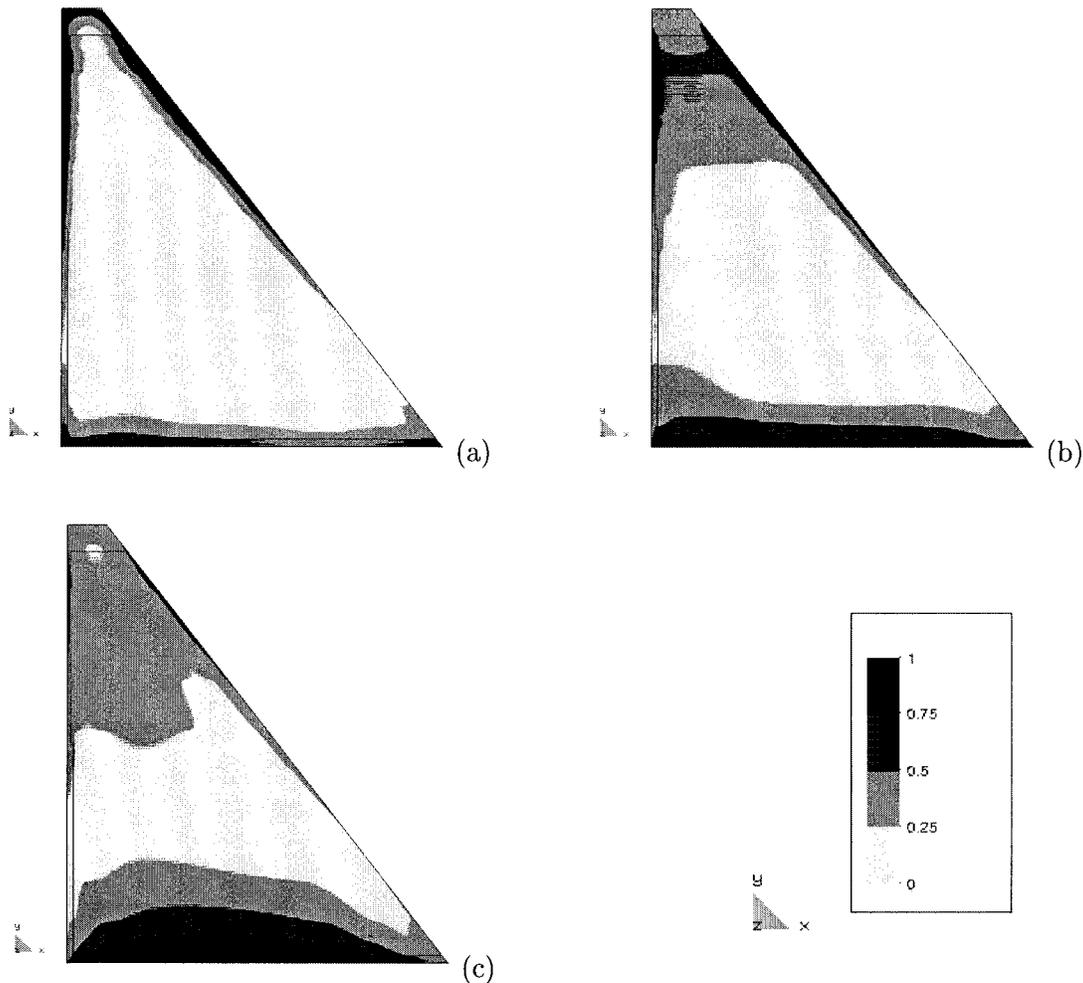
FIG. 6. Long-Term Evolution of Tensile Ratio; Winter Distribution for: (a) 1989; (b) 1991; (c) 1999
