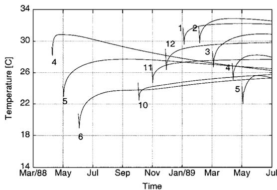
FIG. 7. Temperature Evolution for Different Elevations with 3-Month Interruption
