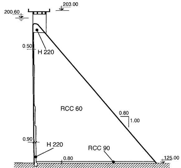
FIG. 2. Cross Section of Urugua-í Dam
