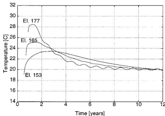
FIG. 7. Long-Term Temperature Evolution for Different Elevations
