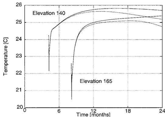
FIG. 9. Long-Term Temperature Evolution for Different Elevations Computed Using 1D (Solid Line) and 2D (Dashed Line) Models
