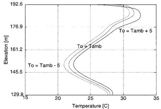
FIG. 10. Influence of Placing Temperature
