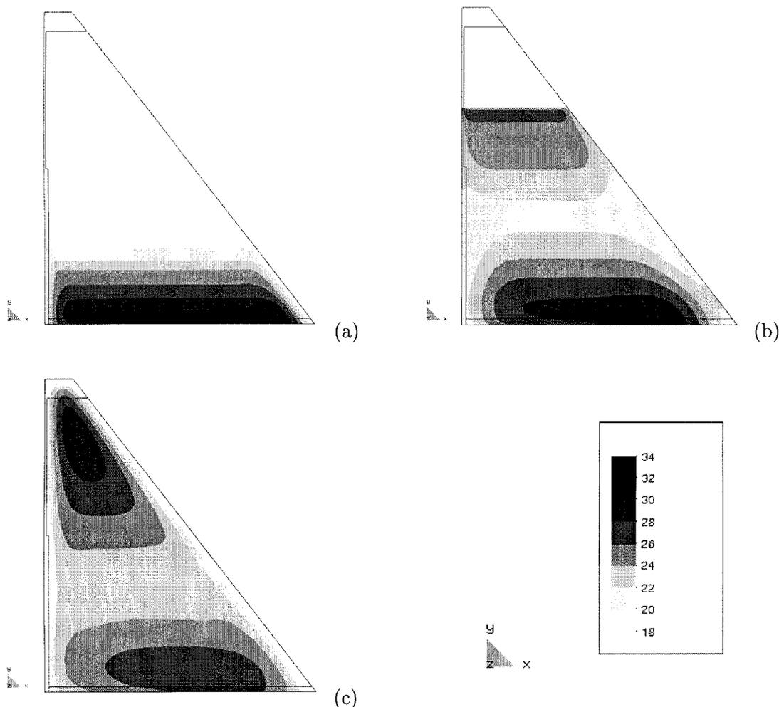
FIG. 5. Short-Term Evolution of Temperatures (°C); Corresponding (Months) Elevations Are: (a) (June 1988) 146 m; (b) (November 1988) 175 m; (c) (June 1989) 196 m
