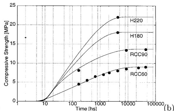
FIG. 1. Comparison with Experimental Data: (a) Temperature Evolution in Adiabatic Tests; (b) Strength Evolution in Isothermal Tests
