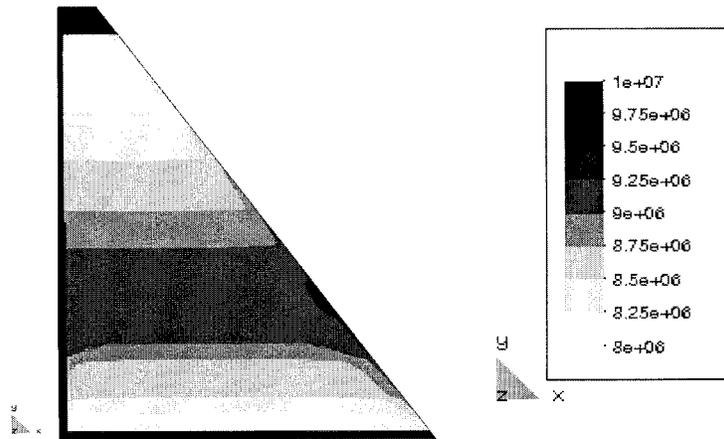
FIG. 6. Distribution of Compressive Strength (MPa) at Completion of Dam (1 Year)
