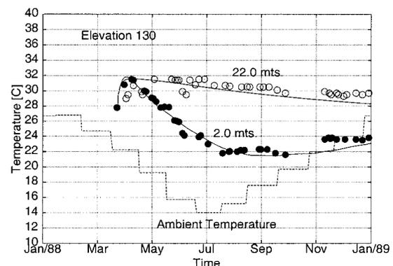
FIG. 3. Comparison between Computed and Measured Temperature Evolution in Dam
