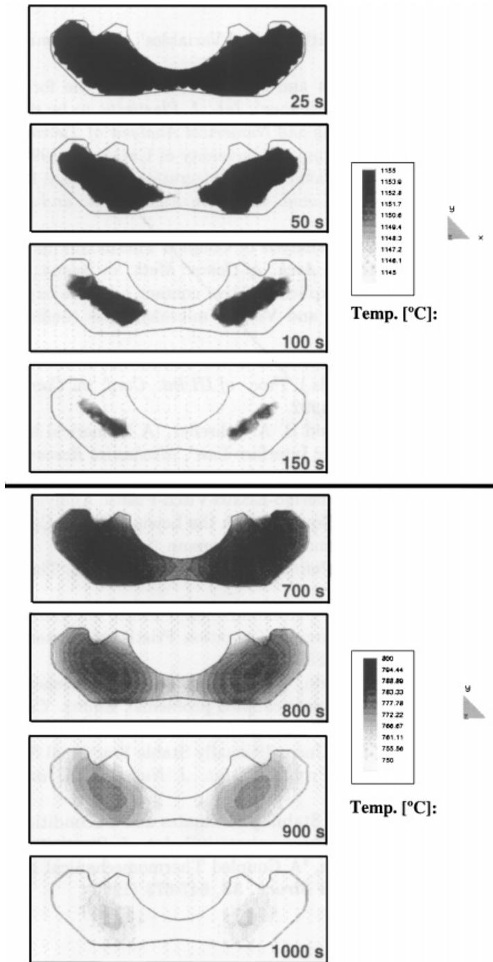
Figure 8. Solidification of a brake component. Evolution of the phase changes on section  $x-y$
