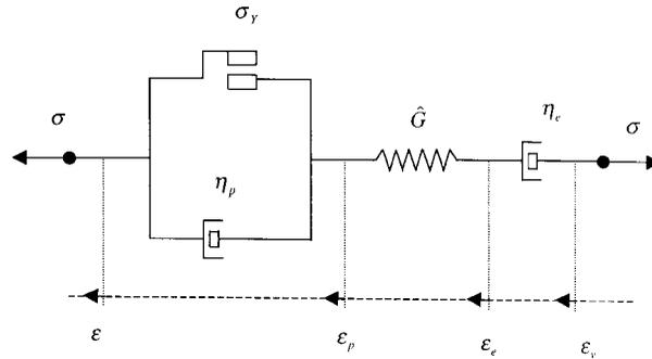
Figure 1. Rheological mechanical model with phase change
