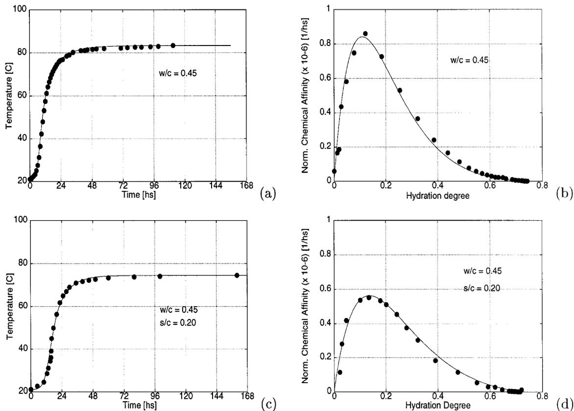
FIG. 1. Temperature Evolution and Normalized Affinity for Adiabatic Tests
